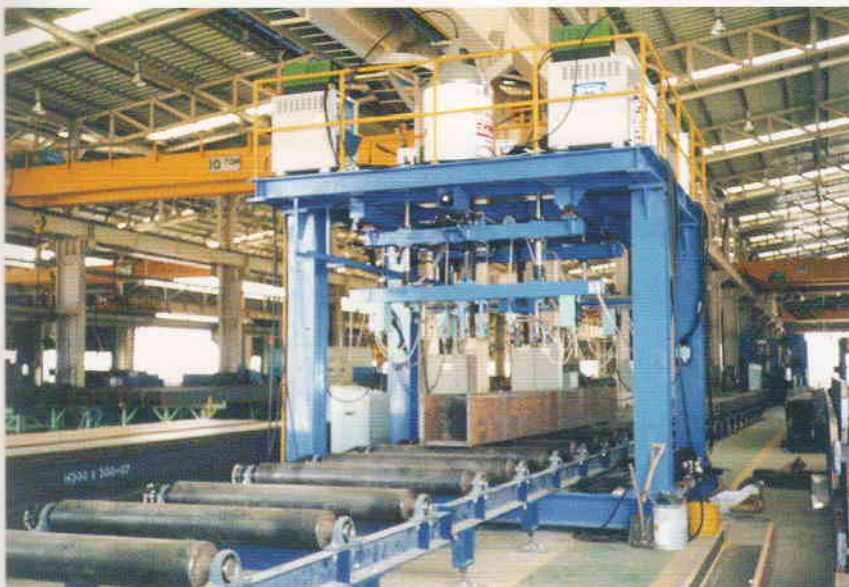
◀ 4 POLE SESNET (LH+RH×2SETS) MAX. 용접간격 : 3800mm
