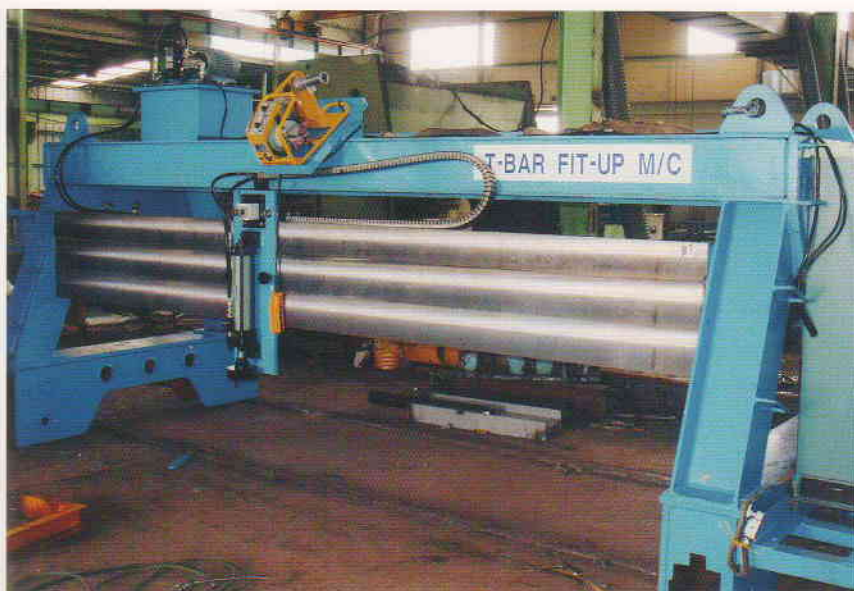
◀ ONE HEAD Type 가압력 7TON LINE SPEED : 15 m/min
